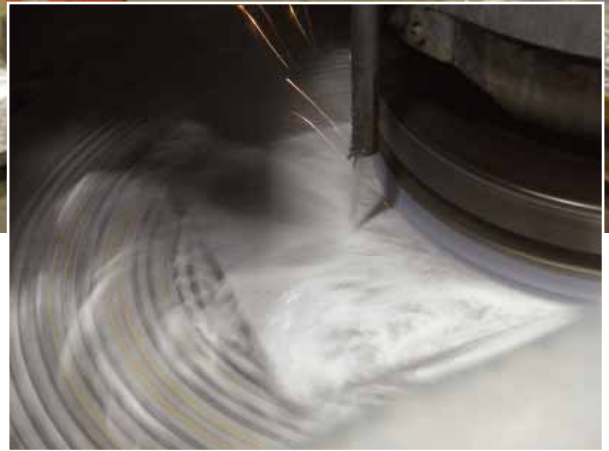
Blanchard Grinding High horsepower rotary grinders quickly and efficiently remove large amounts of stock.
