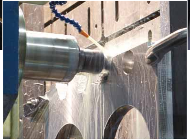
Horizontal Milling This horizontal ground boring machine is creating a series of slots in a large steel part.
